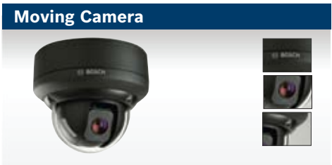
VEZ-211-ICCS SAP NO: F.01U.121.945 Description: High Speed Moving Analog Camera (PTZ), 10x optical Zoom, vandal resistant housing
