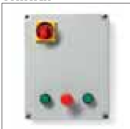
START/THINK control units with open, close, stop buttons with self-hold and three-pole door-blocking switch incorporated in the control panel. Resistant box for use in industrial environments, degree of protection IP 55. Technical features on page 151
